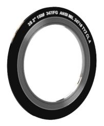
**Style GS (TY2)** comprises of the metal wire with designated filler incorporating the use of a solid metal outer ring. The outer guide ring promotes the correct centering of the gasket in a standard flange, offers radial support for the outer portion of the spiral wound, and acts as compression gauge to prevent over compression of the spiral wound.
